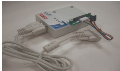
Serial Programming Mode - using EIC-101 Connector
